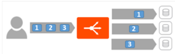
With multiplexing: Request distribution from traffic originating from one client connection
