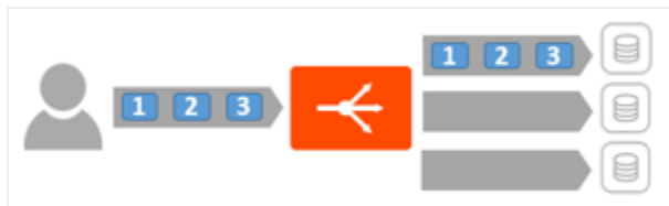
Without multiplexing: Request distribution from traffic originating from one client connection
